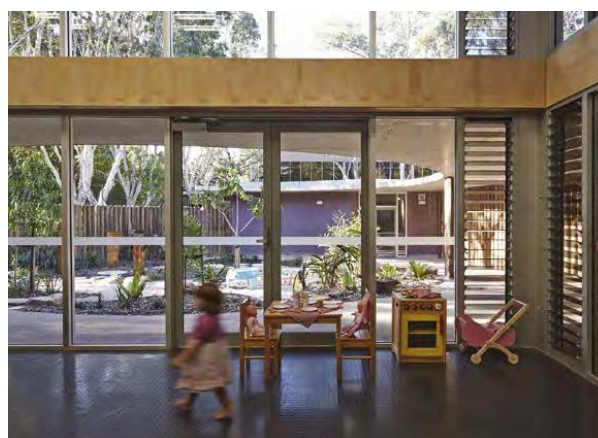
Louvres can be incorporated to allow for ventilation when doors are closed.
